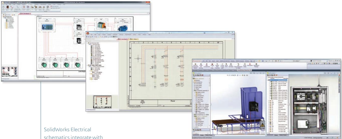
SolidWorks Electrical schematics integrate with SolidWorks 3D models to enable true concurrent electromechanical design.
